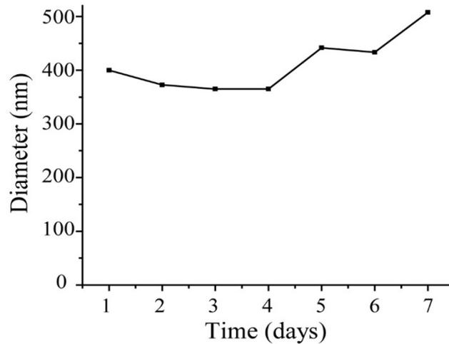
Figure S7. Dynamic light scattering (DLS) data of FLAME-RGD over the course of seven days at 25°C. The slight growth of the average hydrodynamic diameter may be due to the slight
