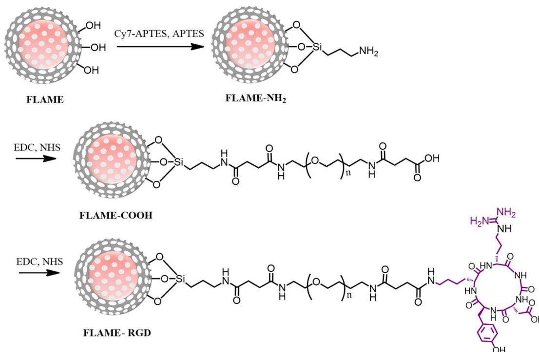
Scheme S2. Synthetic scheme of FLAME-RGD
