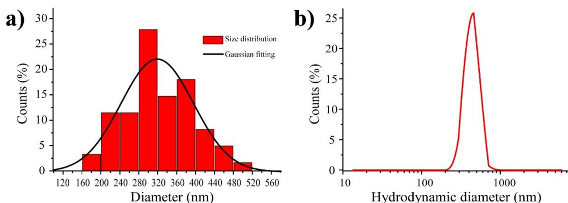
Figure S3. a) size distribution and gaussian fitting of FLAME by transmission electron microscopy (TEM). The average diameter of FLAME is 325 nm and the Standard deviation is 73 nm. b) Hydrodynamic diameter of the FLAME by Dynamic light scattering (DLS), the average hydrodynamic diameter of FLAME is 396 nm.
