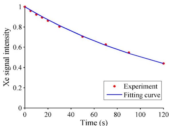
Figure S5. Longitudinal relaxation rates  $R_1^a$  of  $^{129}\text{Xe}$  in solution. The  $R_1^a$  value of  $0.0069 \text{ s}^{-1}$  was measured by fitting the experimental data to equation 1.
